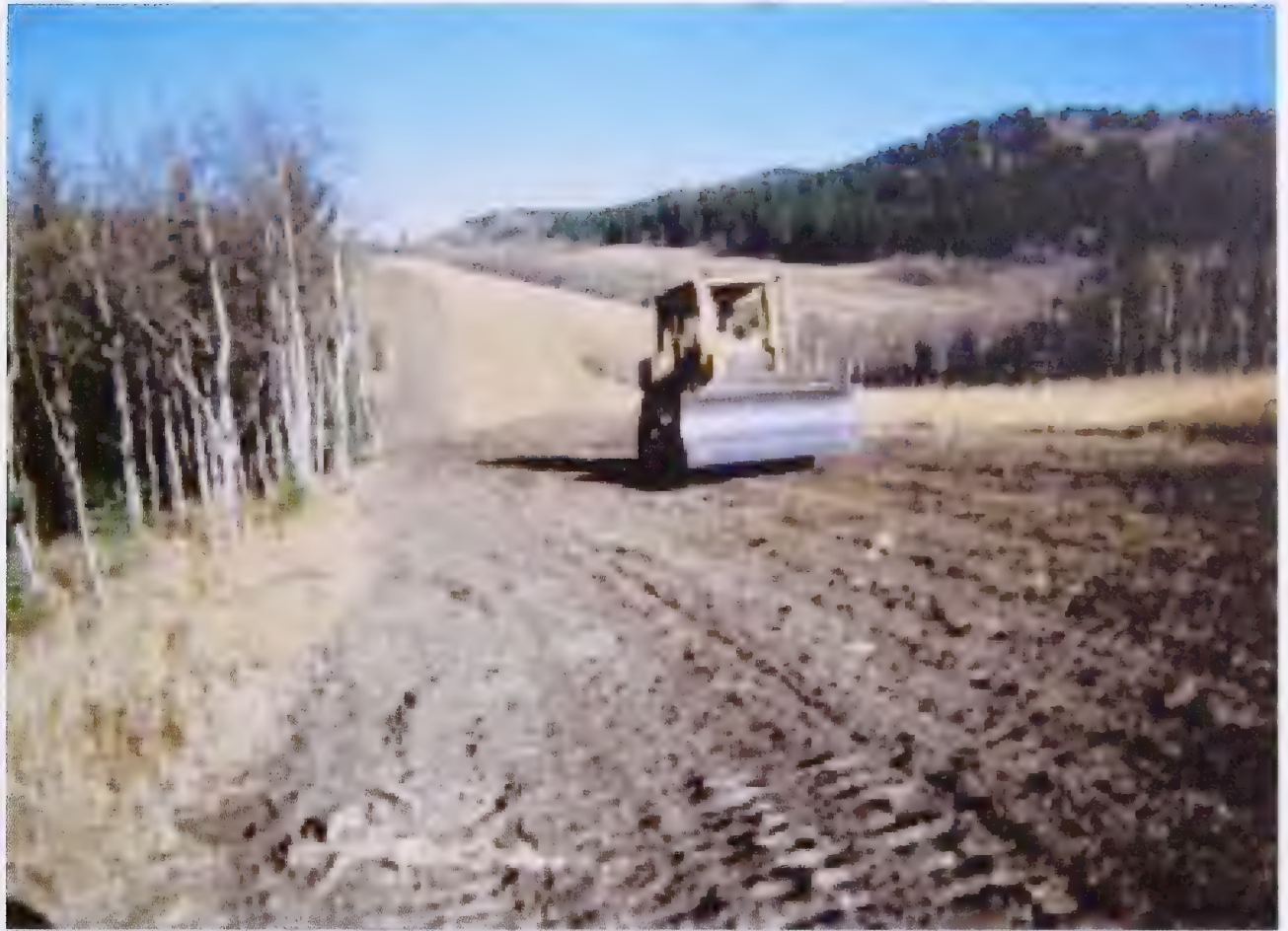
Photo 43 A dozer is used to firm the seed bed and imprint the surface of the soil following seeding operations.
